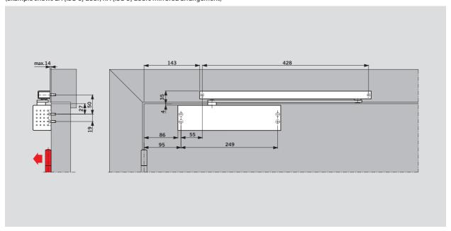
Provided the structural conditions allow, an opening angle of 180° is possible with this method of fixing. In most cases, however, a wall recess will have to be provided for the door closer.
