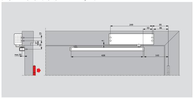
Depending on the structural conditions, the door opening angle with this method of fixing is limited to approx. 120° to 145°. In order to avoid damage to the door or door closer, users are recommended to install a cushioned backstay or a door stop.
