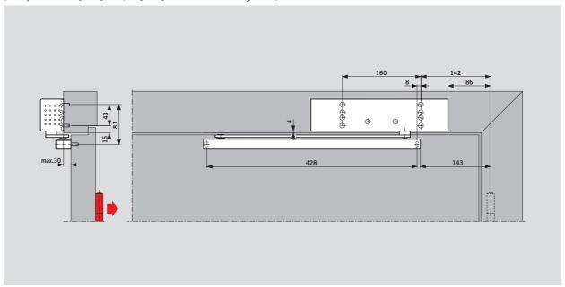
Depending on the structural conditions, the door opening angle with this method of fixing is limited to approx. 120° to 145°. In order to avoid damage to the door or door closer, users are recommended to install a cushioned backstay or a door stop.
