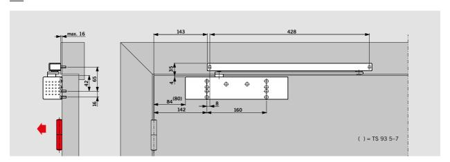
Door leaf fixing (standard arrangement) of the TS 93 B on the pull side. Structural conditions permitting, an opening angle of 180° is possible with this fixing method. In most cases, a wall recess may have to be provided for the door closer.
