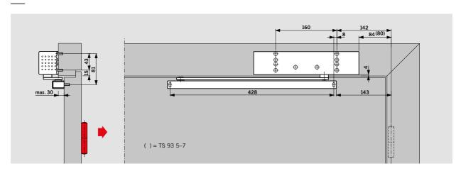
Transom fixing (overhead frame fixing) of the TS 93 B on the push side. Backcheck and delayed action non-operative with this fixing arrangement. The door opening angle is limited to approx. 120° to 145°,
